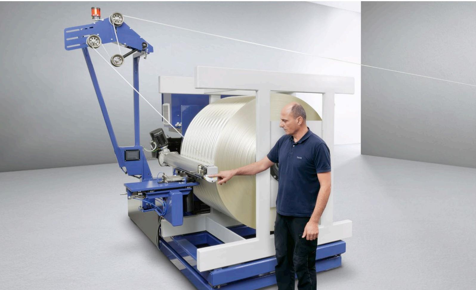
The **T1 RackWinder** is part of the revolutionary SAHM T1 System that reduces downtime in your carbon fiber processes and increases production efficiency by up to 92 %. The T1 RackWinder winds the sensitive precursor material with high precision into bobbins of up to one ton.
