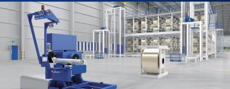
The SAHM T1 System is a completely new concept for handling materials in upstream carbon fiber processes. It uses bobbins with one ton of precursor material which results in significantly fewer oven stops, making it possible to achieve a tripling of production output while at the same time reducing waste.
