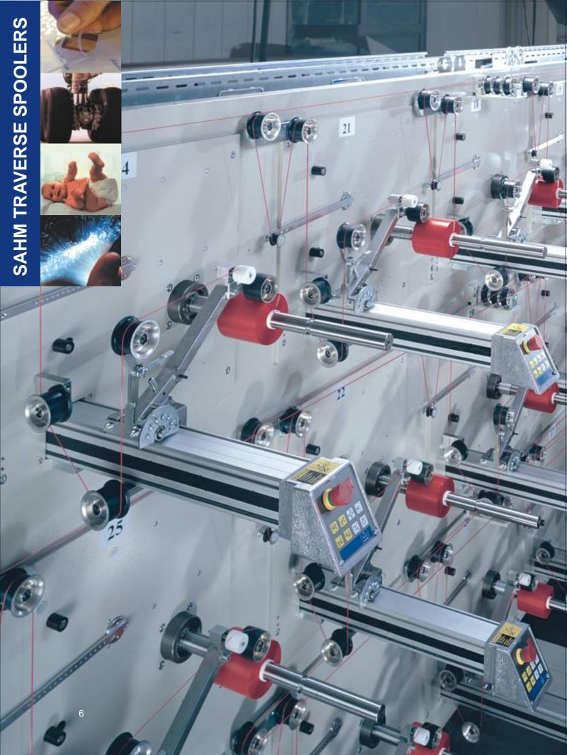
Continuous operation of production lines requires greater lengths. This can be achieved with our traverse winders. Depending on the physical properties of the materials, many thousand meters can now be traverse wound on a tube or spool.
